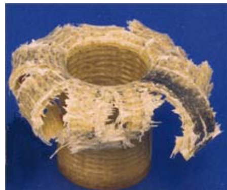
Figure 2. Sample failure mechanisms in a cross-ply stitch mat composite tube. Specimens and photographs are courtesy of the Automotive Composites Consortium.
