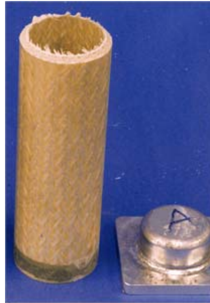
Figure 1. Typical metallic crush initiator and beveled composite tube. Specimens and photographs are courtesy of the Automotive Composites Consortium.
