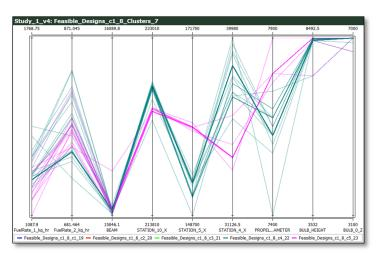
IMAGE ON LEFT - Result of a cluster analysis on a 2D relation plot to identify the designs with high performance metric. IMAGE ON RIGHT - Results of a clustering analysis on the "good designs" identified in the previous analysis to identify any trends in the variable space. The results show two slightly different design concepts that give similar results in terms of design performance.
