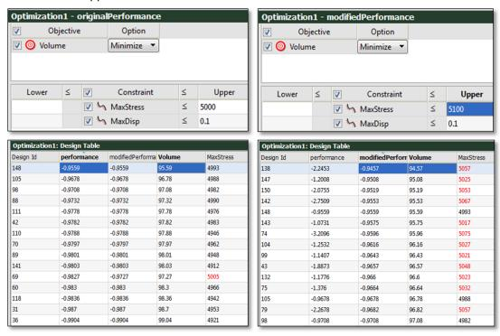
The figures above show the original and the new modified performance definitions. The design tables show the designs sorted using the performance definition above the table. You can see that with the relaxed constraint in the modified performance, there is a design in the existing set with a lower volume.
