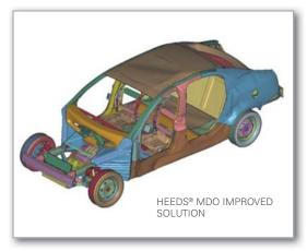
The optimization reduced the mass of the designed parts by 33.5kg. This resulted in a reduction of 22% over the baseline design (from 152 to 118.5kg). The relative cost measure was also reduced by 19%.
