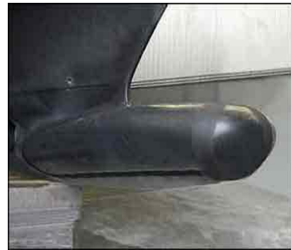
Figure 3 - Bulbous bow with thermo-formed OceaPoly protective surface.
