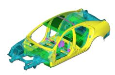
ETA's ACP process uses innovative, holistic product development process with multi-disciplinary (MD) loading based on topology and 3G (geometry, grade, and gage) optimization. It incorporates Red Cedar Technology, Inc.'s HEEDS® Professional (<a href="http://www.redcedartech.com">http://www.redcedartech.com</a>), a powerful software package that automates the design optimization
