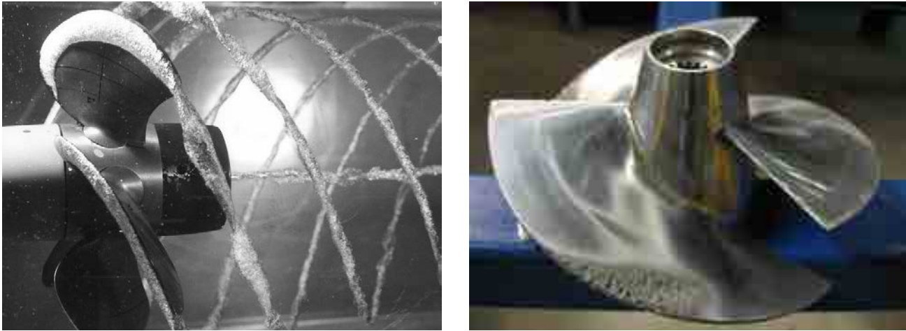
FIGURE 4: Tip vortex and blade back cavitation (left), and cavitation damage (right)
